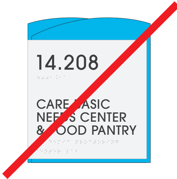
AVOID BACK-TO-BACK MOUNTED SIGNS ON GLASS FROM HAVING COMPETING ARCHES VISIBLE
