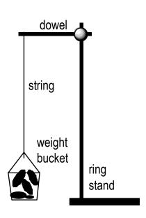
apparatus consists of a ring stand, a wooden dowel attached to the ring stand by means of a lamp, a string with one end attached to the end of the dowel and the other end attached to a small bucket, and gravel to be used to add weight to the bucket. The instructor will discuss the basic use of the pendulum, including how to change some of the variables, such as weight and length.
