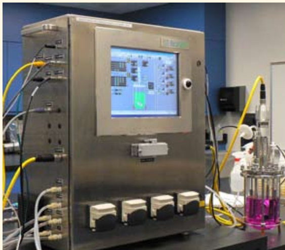
State-of-the-art DeltaV digital bioreactor control system
